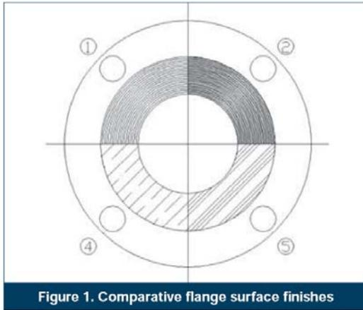
Figure 1. Comparative flange surface finishes
