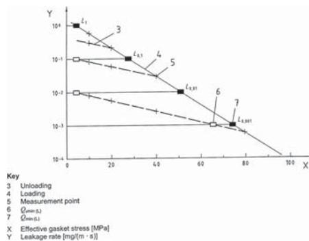
Figure 2. Leakage rate as a function of gasket stress (for an internal pressure of 40 bar in this case).
