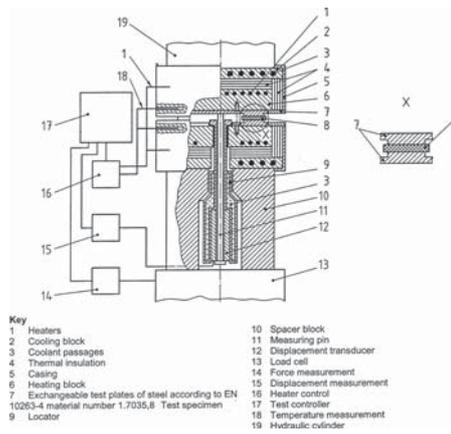
Figure 1. Test rig schematic for compression, compression creep and creep relaxation tests.
