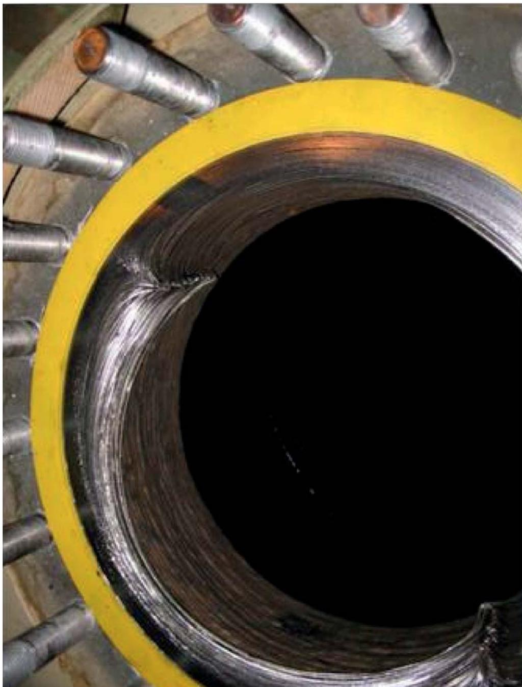
*spiral wound gasket; sealing element with outer ring only. Failure: mode inner ring buckling. Cause: incorrect size\no inner support ring*
