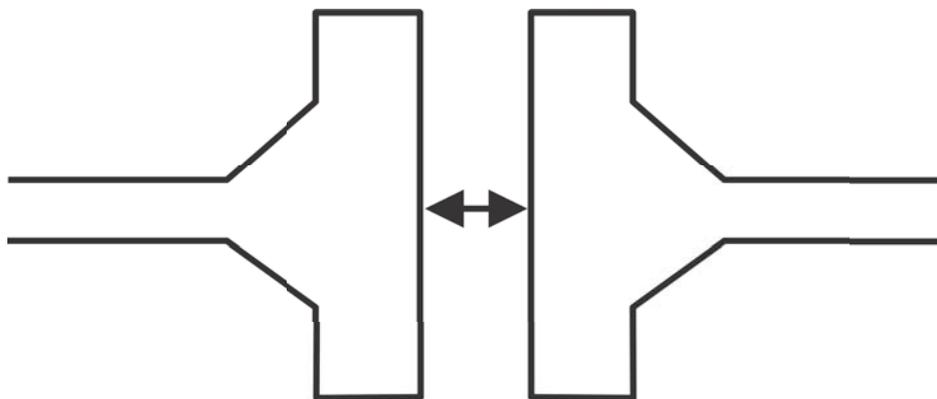
Fig. E-4 Excessive Spacing or Gap
