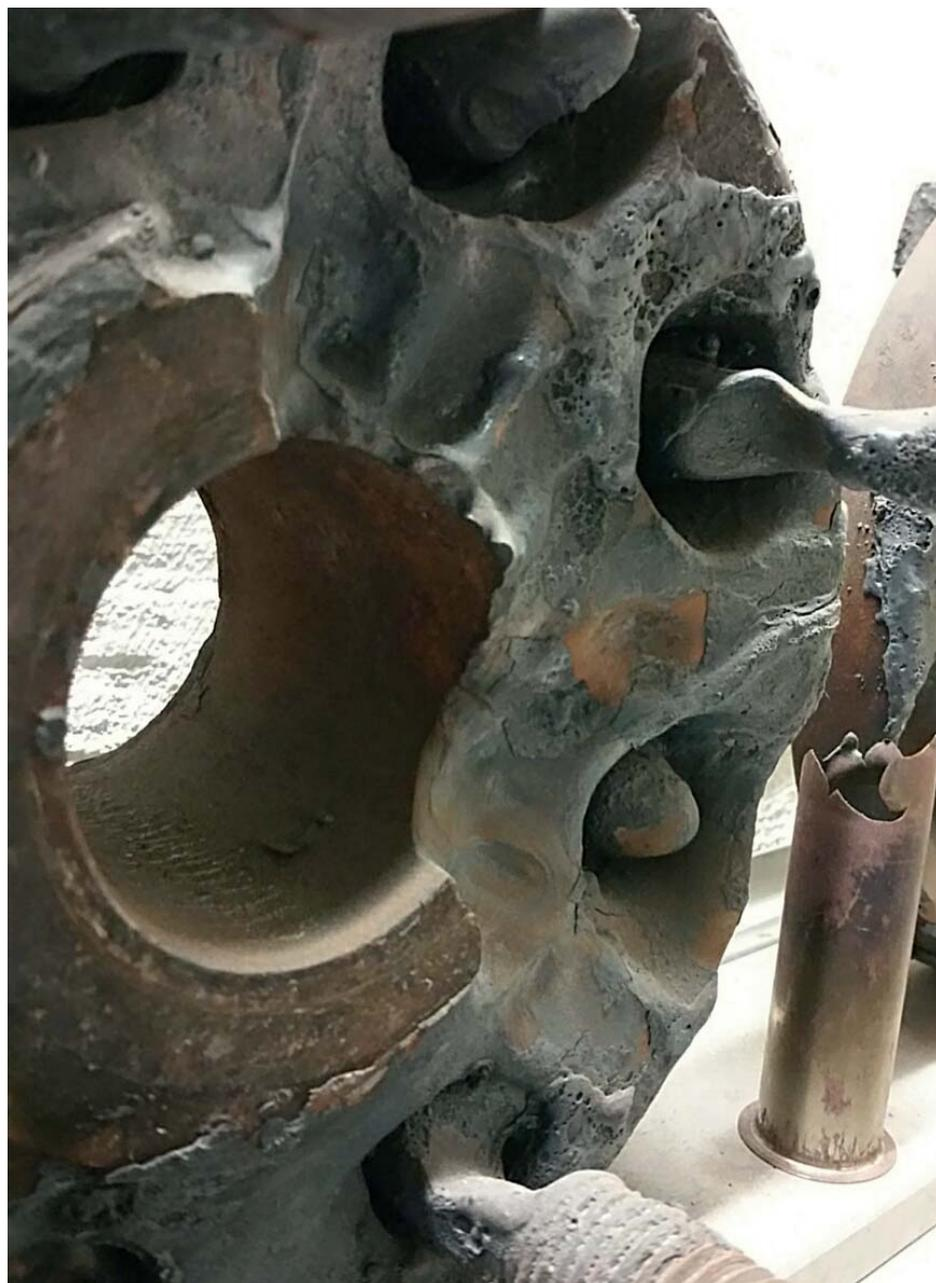
*Flange severely damaged by ignition in oxygen.*
