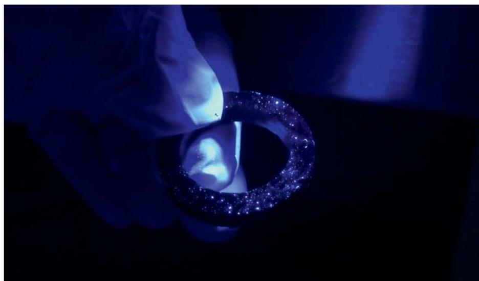
*Packing ring under UV light showing particulate contamination – a potential source of ignition.*
