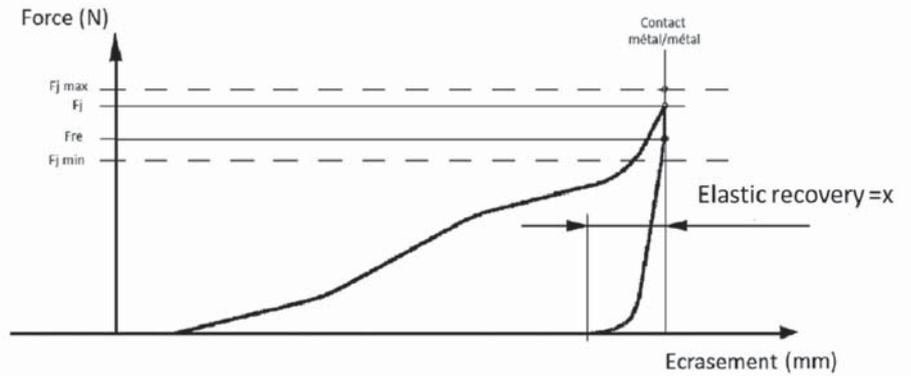
Figure 7. Load as a function of the thickness of the gasket (Source: EDF specification)
