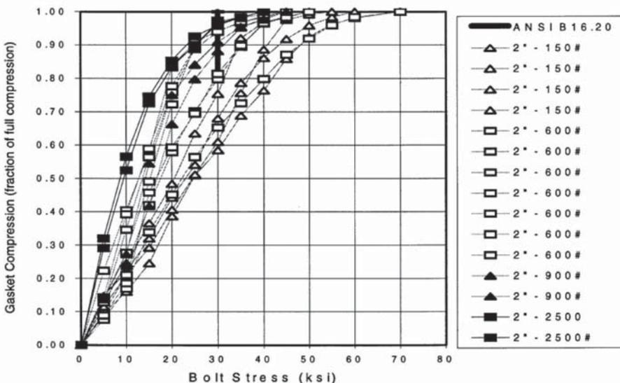
Figure 6. Load-deflection characteristics of fifteen 2-inch spiral-wound gaskets
