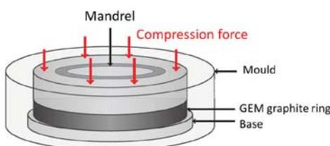
Figure 1. Tooling schematic for graphite ring production
