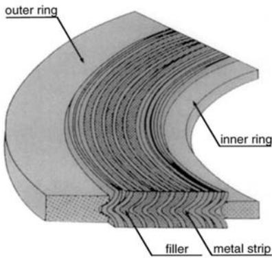
Figure 5. Configuration of a spiral wound gasket
