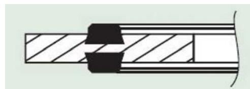
Figure 2. GEM gasket design with grooves
