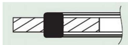
Figure 3. GEM gasket design with two metal rings
