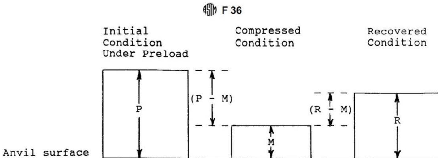
FIG. 1 Representation of Specimen Thickness
