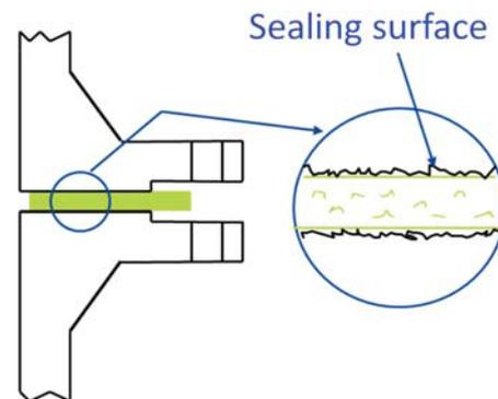
Figure 1: Surface structure of the sealing surface.
