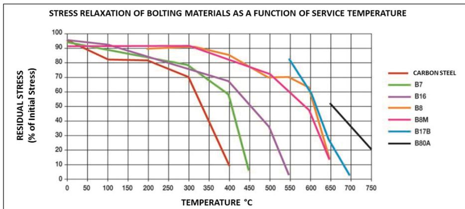
The creep of bolting can be seen in the graph below showing the residual stress in different common bolting material after 1000hr of exposure to different temperatures.
