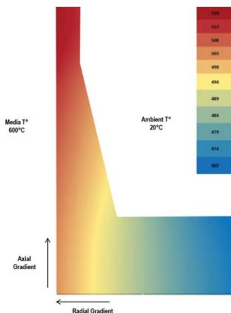
Again, effects of temperature on bolts and flanges assembly are not addressed by the traditional “Taylor Forge” calculation, other than the impact on the material stress limit. EN1591 has made significant improvement introducing assessment of differential axial thermal expansion between the bolts and the flanges. As an example, in the French code – CODAP – the differential axial thermal expansion is not addressed and said to be negligible if:
