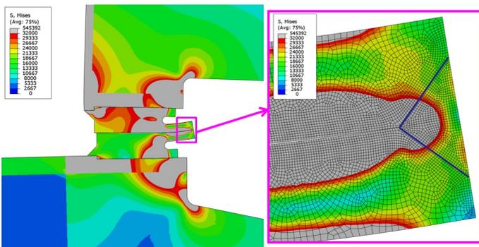
**Figure 14. Contours of Elastic von Mises Stress (psi) in the Flat-Lip Weld Ring Gaskets and Seal Weld Under Operating Loads.**
