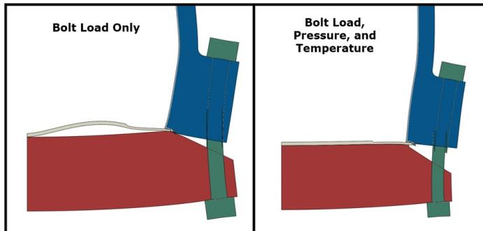
Figure 25. Deflections in the Original Channel Cover Diaphragm Seal Assembly Due to Preload and Operating Loads (Deformation Scale Factor = 100).
