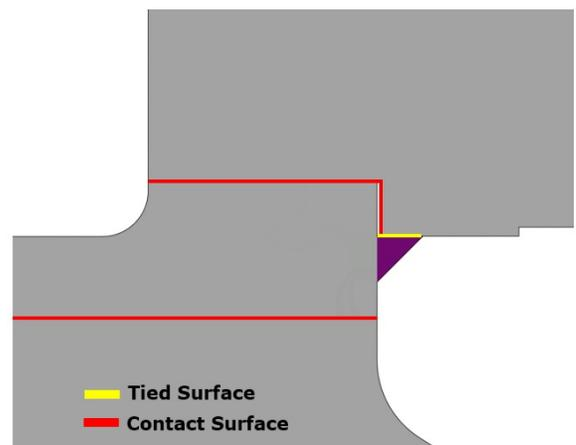
Figure 10. Contact and Tied Surfaces in the FEA Model with the Original Diaphragm Seal Design.
