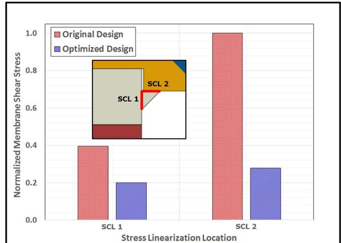
Figure 29. Comparison of Normalized Membrane (Average) Shear Stress in the Diaphragm Seal Weld for the Original and Optimized Designs.
