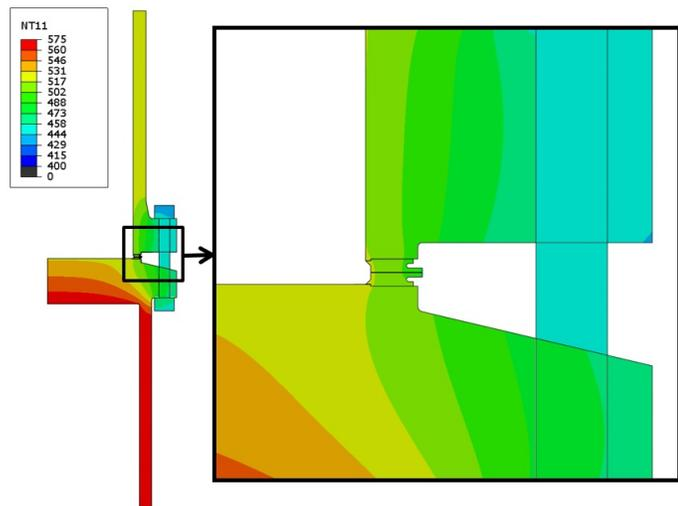
Figure 11. Steady-State Temperature Distributions (°F) in the Original Weld Ring Gasket FEA Model.
