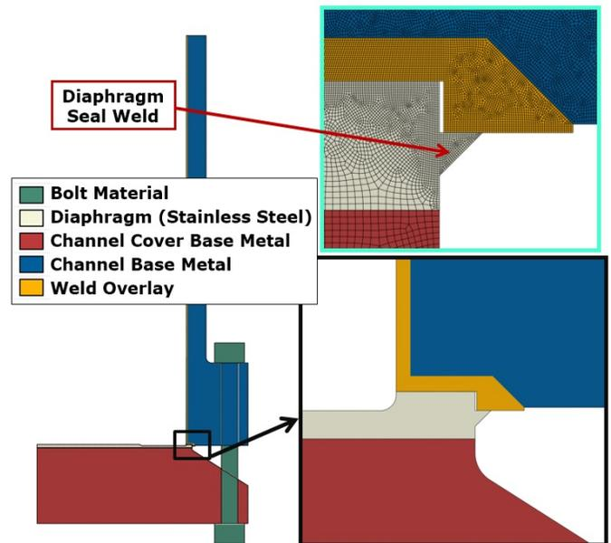
Figure 9. Axisymmetric FEA Model of the Channel Shell-to-Channel Cover Flanged Joint with the Original Diaphragm Seal Design.
