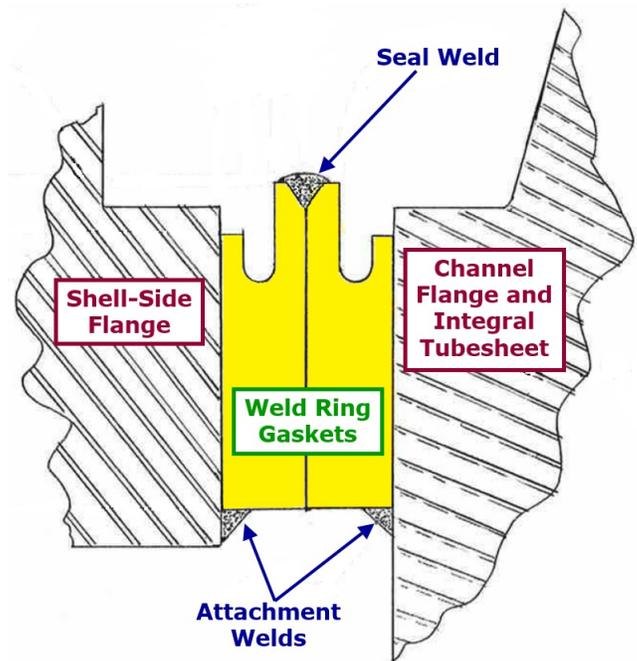
Figure 2. Sketch of the Flat-Lip Seal Weld Ring Gasket Configuration that Leaked In-Service.
