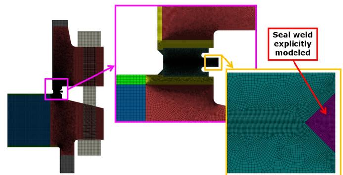
Figure 6. Mesh Refinement of the Channel-to-Shell-Side Flanged Joint with the Original (Flat-Lip) Weld Ring Gaskets.
