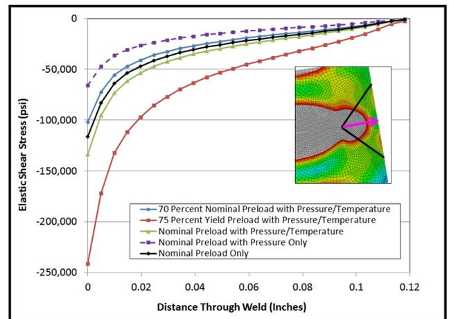
**Figure 15. Through-Thickness Elastic Shear Stress in the Flat-Lip Weld Ring Gasket Seal Weld For Different Load Cases.**
