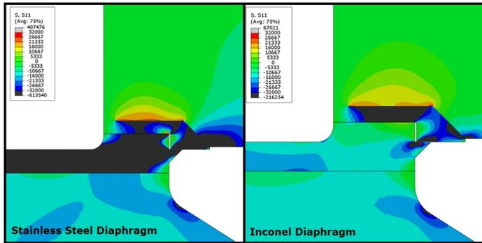
Figure 27. Contours of Radial Stresses (psi) in the Diaphragm Seal Assembly with Stainless Steel and Inconel Diaphragms.
