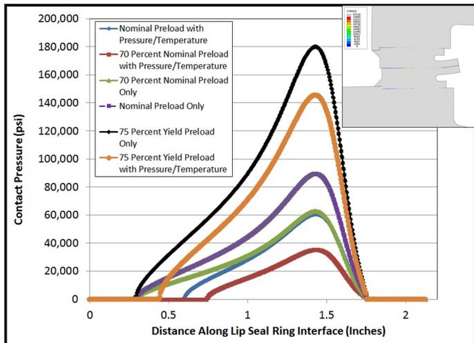
Figure 16. Contact Pressure (psi) Across the Face of the Weld Ring Gasket Interface For Different Load Cases.
