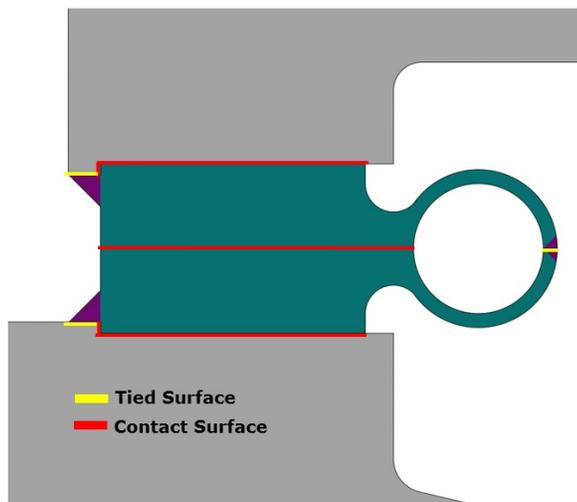
Figure 8. Contact and Tied Surfaces in the FEA Model with Modified Hollow-Lip (Omega) Weld Ring Gaskets.
