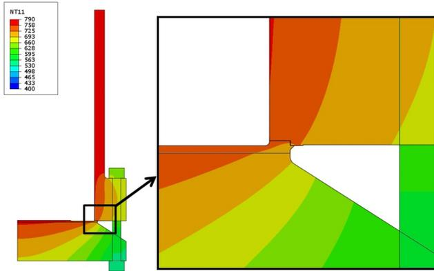
Figure 24. Steady-State Temperature Distributions ( $^{\circ}$ F) in the Original Channel Cover Diaphragm Seal FEA Model.
