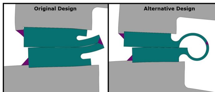
Figure 18. Deflections Due to Bolt Load for Original (Flat-Lip) and Alternative (Hollow-Lip) Designs (Deformation Scale Factor = 25).
