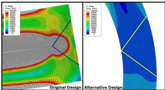
**Figure 19. Contours of Elastic von Mises Stress (psi) in the Original and Alternative Design Seal Welds Under Operating Loads.**
