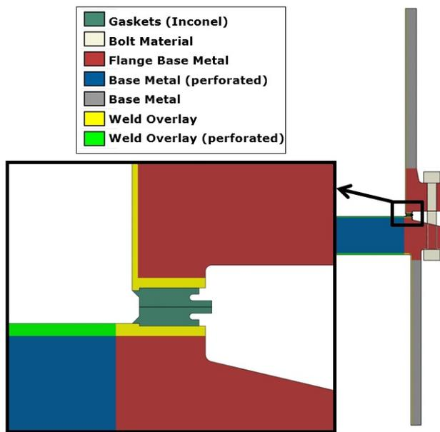
Figure 5. Axisymmetric FEA Model of the Channel-to-Shell-Side Flanged Joint with the Original (Flat-Lip) Weld Ring Gaskets.
