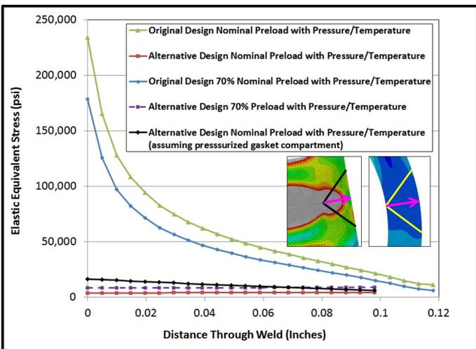
**Figure 20. Elastic von Mises Stress (psi) Through the Original and Alternative Design Seal Welds For Different Load Cases.**
