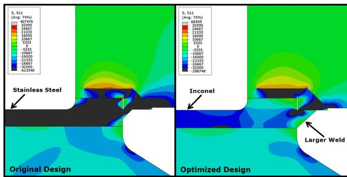
Figure 28. Contours of Radial Stresses (psi) in the Diaphragm Seal Assembly for the Original and Optimized Designs.
