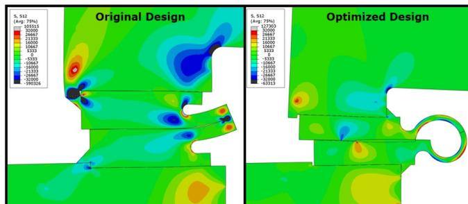
**Figure 22. Contours of Elastic Shears Stress (psi) in the Original and Optimized Gasket Designs (Deformation Scale Factor = 10).**
