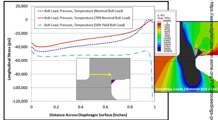
Figure 26. Compressive Stress (psi) in the Diaphragm Gasket for Varying Amounts of Bolt Load.
