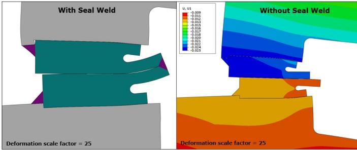
**Figure 13. Deflections with the Seal Weld Modeled and Contours of Radial Deflections (inches) with Seal Weld Removed for Bolt Load.**
