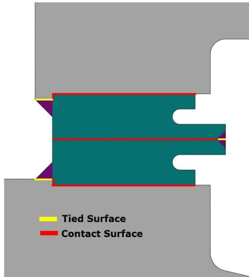
Figure 7. Contact and Tied Surfaces in the FEA Model with the Original (Flat-Lip) Weld Ring Gaskets.
