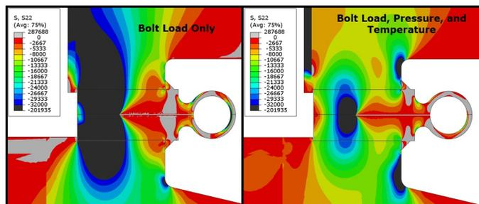
**Figure 23. Contours of Elastic Longitudinal (Compressive) Stress (psi) in the Optimized Gasket Design for Bolt and Operating Loads.**
