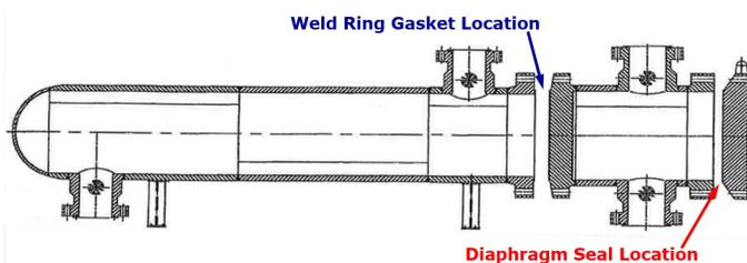
**Figure 4. Simplified General Layout Drawing of Heat Exchanger Evaluated Herein.**
