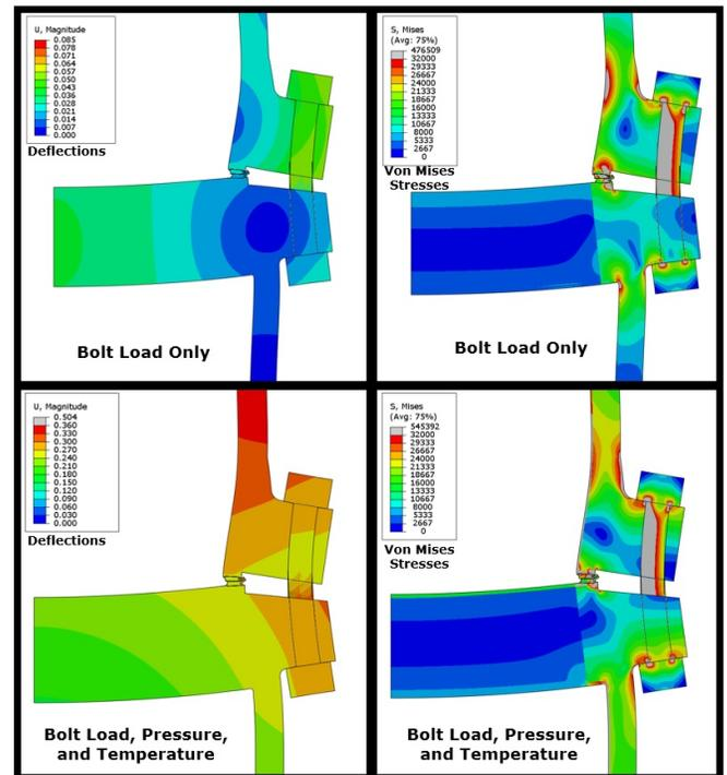
Figure 12. Deflections (in inches) and von Mises Stress (in psi) for Bolt Loading and Operating Loads (Deformation Scale Factor = 50).
