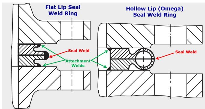
Figure 1. Sketches of Flat and Hollow-Lip (Omega) Seal Weld Ring Gasket Designs.
