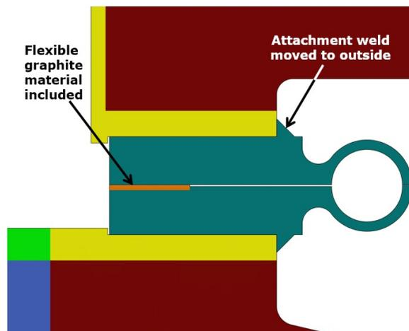
**Figure 21. Optimized Weld Ring Gasket Design with Graphite Material and Relocated Attachment Weld.**
