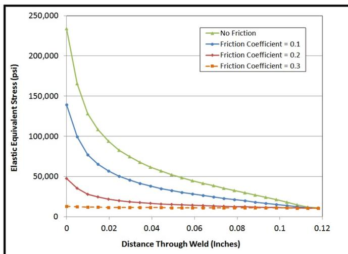
Figure 17. von Mises Stress (psi) Through the Flat-Lip Seal Weld for Varying Friction Coefficients.
