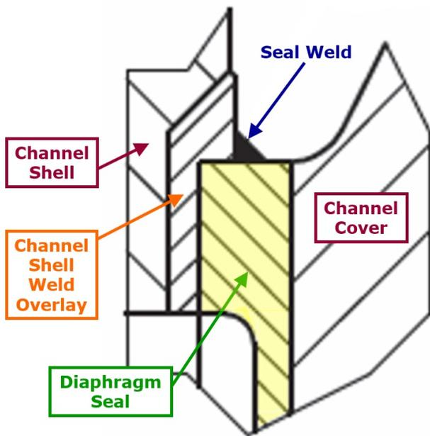
**Figure 3. Original Channel Cover Diaphragm Seal Configuration with Seal Weld.**
