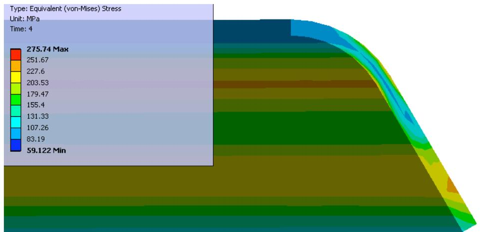
Fig. 9. Stresses reduced in the modified gasket upper layer
