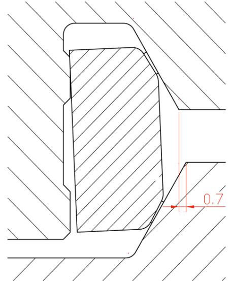
Fig. 7. Gasket in operating condition
