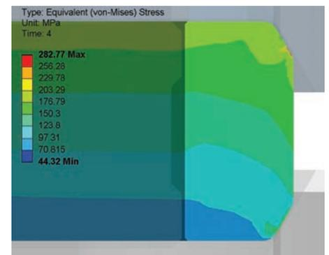
Fig. 4. Stresses reduced in the gasket
