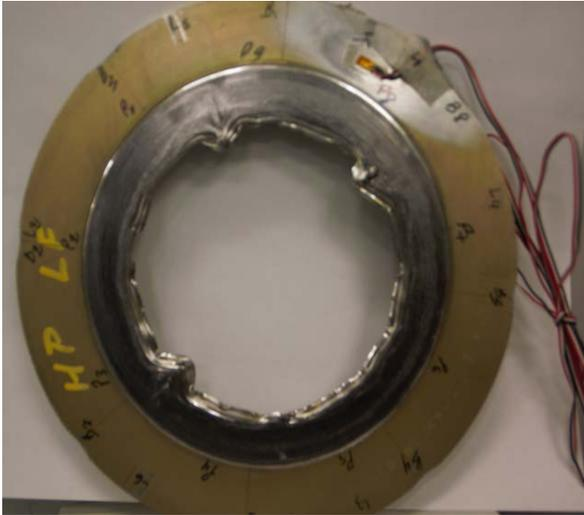
**Figure 10:** SW gasket showing buckled windings
