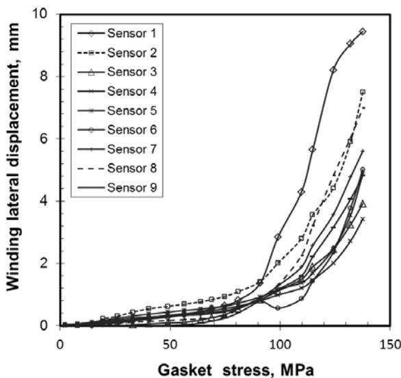
**Figure 11:** Winding inward radial displacement as a function of gasket compressive stress
