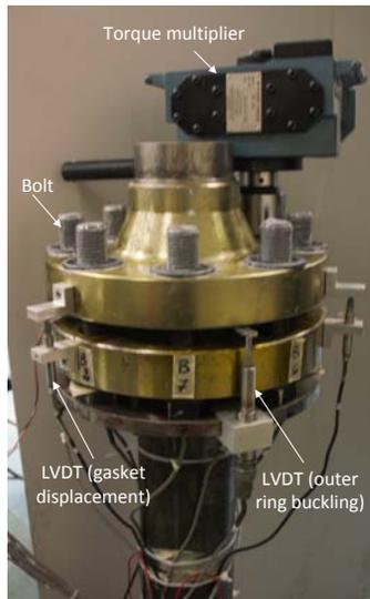
**Figure 2** Instrumented NPS 4 class 900 bolted joint
