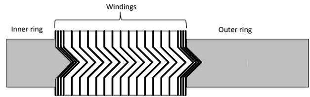
**Figure 1:** Spiral wound gasket with outer ring
