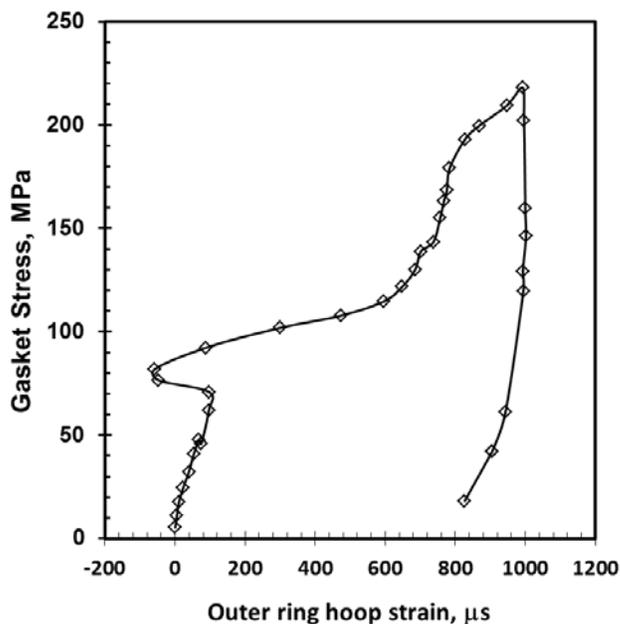
**Figure 9:** Measured outer ring Hoop strain
