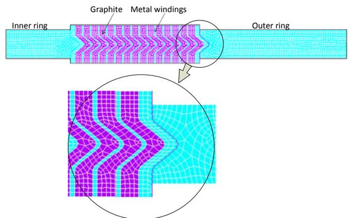
**Figure 4** FE mesh model of a SW gasket
