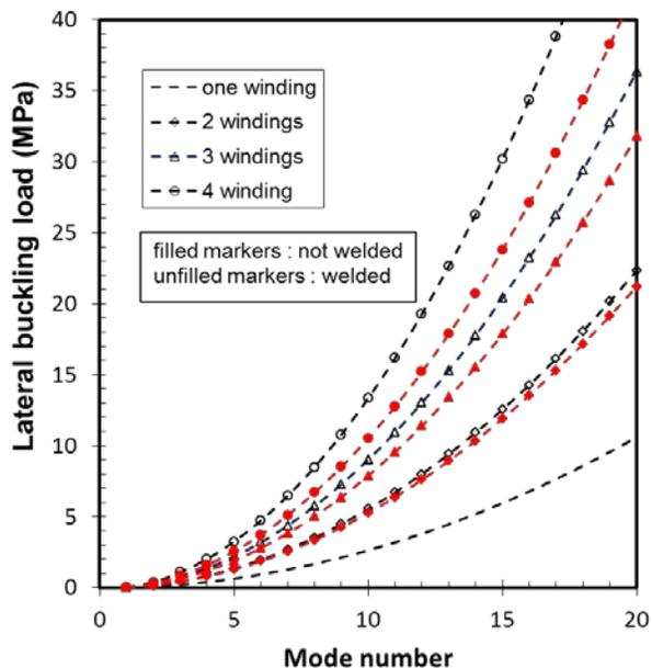
**Figure 7:** Relationship between load and windings
