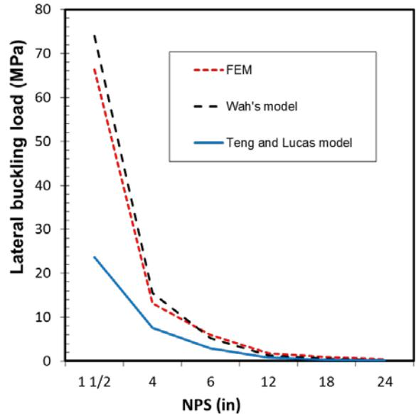
Figure 5: Buckling of inner ring of class 900 SW gaskets: Analytical and numerical FE results
