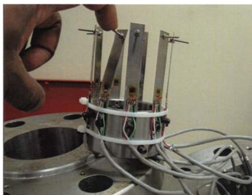
**Figure 3:** Inward radial displacement sensor
