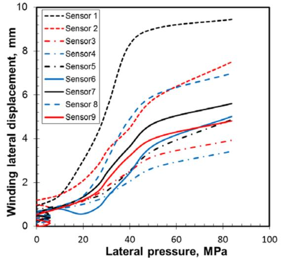
**Figure 12** Winding inward radial displacement as a function of lateral pressure
